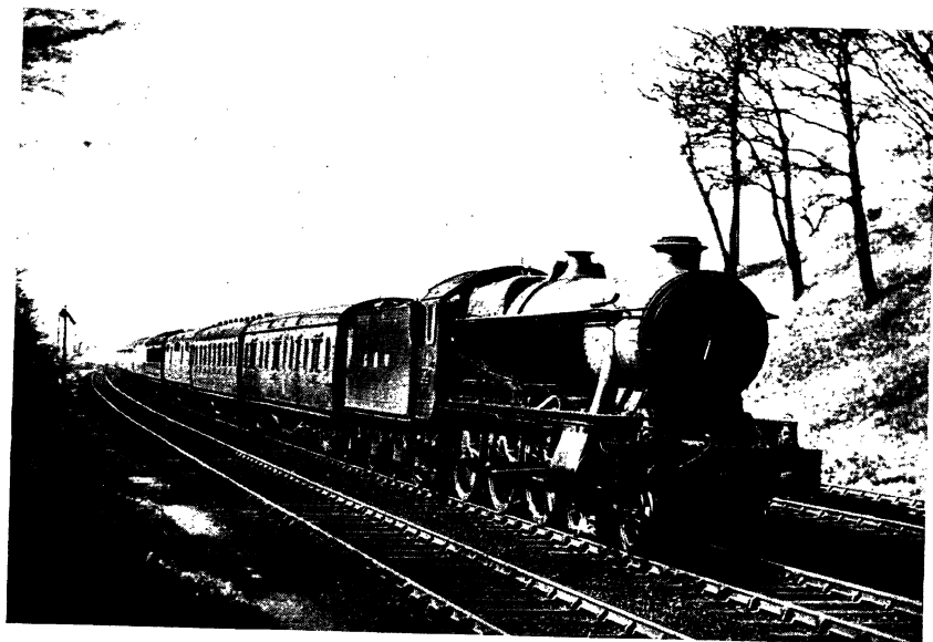
83. A 4-cylinder 4-6-0 of the Churchward "Star" class, precursors of the Collett "Castles." Malmesbury Abbey is being coaled. (M. W. Earley.)
