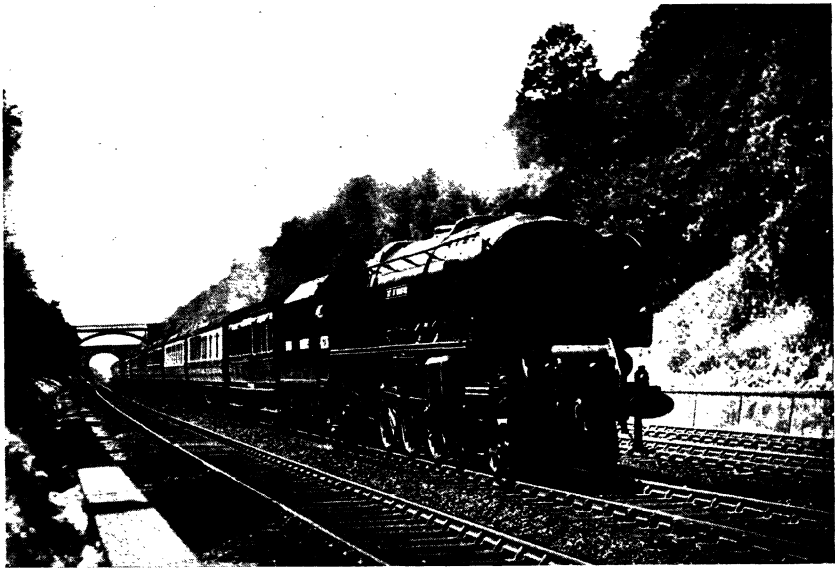
46. At the start of a dynamometer test. The Eastern Region car is at the head of the 1.10 p.m. express from King's Cross in the 1948 exchange trials, and the engine is London Midland Region rebuilt "Royal Scot" Queen's Westminster Rifleman . (F. R. Hebron.)
