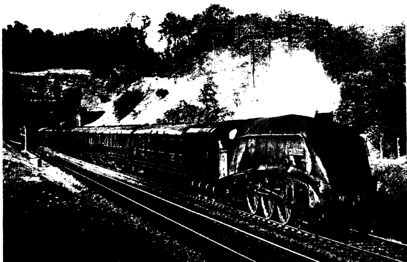
79. Gresley's most successful design— Silver Fox , a Class "A4" streamlined Pacific, making speed near Abbots Ripton with the up "Silver Jubilee." (C. C. B. Herbert.)
