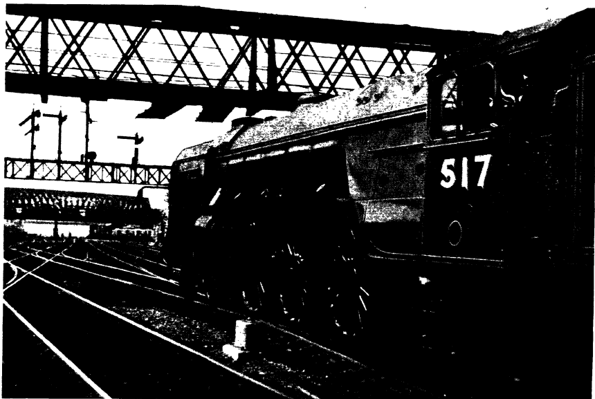
75. One of the Peppercorn 6 ft. 2 in. Pacifics, Trimbush , about to leave King's Cross. Note the electric lighting, with ordinary unlighted lamps carried above for daytime head-code indication. (C. C. B. Herbert.)
