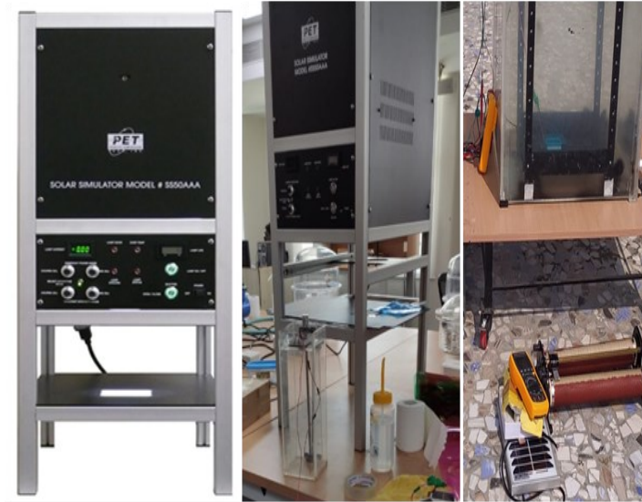
Figure 3.17 a) Solar simulator providing STC b) Experimental setup of monocrystalline solar cell under solar simulator c) Experimental setup of monocrystalline Si cell under sun at 12 PM with >1000 \text{ W/m}^2
