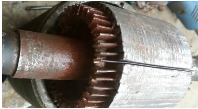
Figure 6.2 Rotor of DFIG with single rotor bar (removable and attached via welding)
