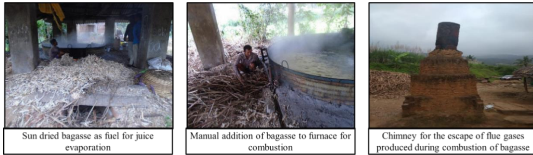
Figure 2.6 Representative pictures of juice evaporation process (Source: field visits at Marayoor, Kerala, India).
