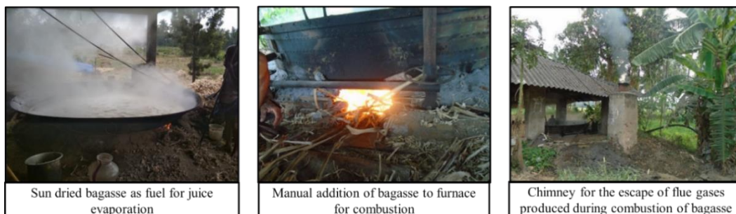
Figure 2.5 Representative pictures of juice evaporation process (Source: field visits at Anakapally, AndhraPradesh, India).
