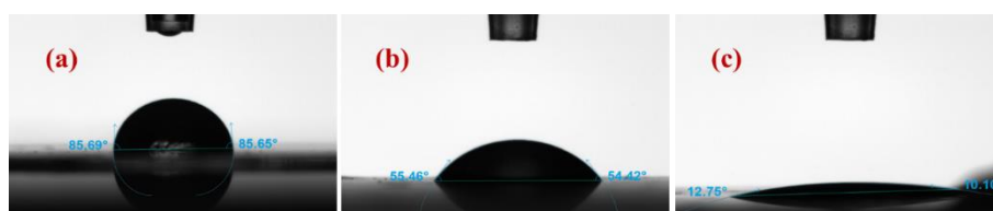
Figure 2.3 Contact angle measurements over (a) pristine, (b) 2 h alkaline hydrolyzed, and (c) 4 h alkaline hydrolyzed PCL films.
