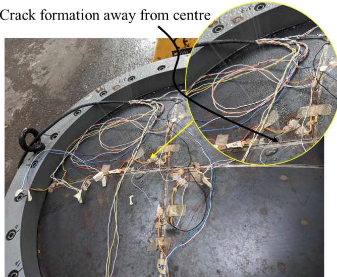
c) Crack initiation during the experiment
