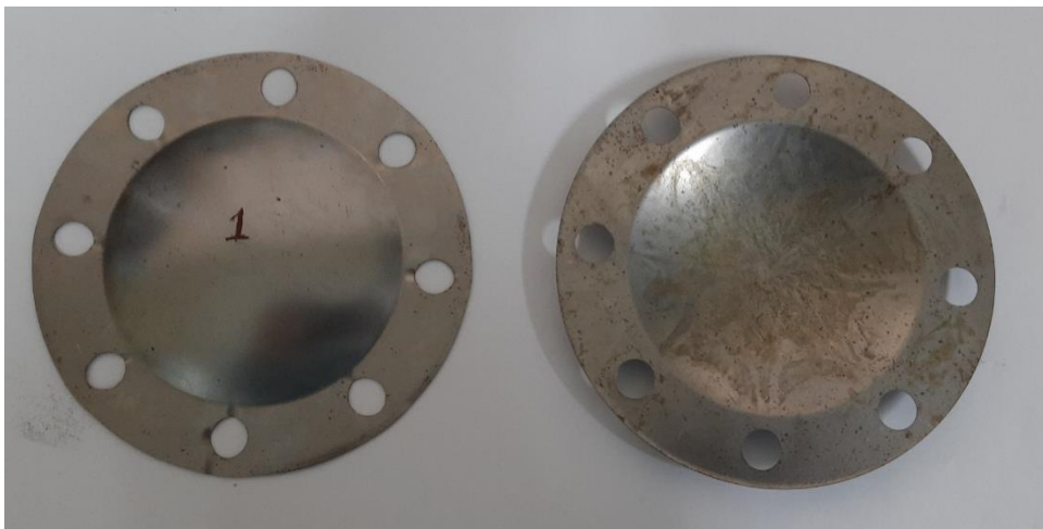
Figure 5.9: Hydro-formed domed GS disc (finished component)
