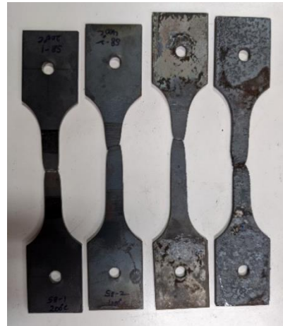
(a) Specimen geometry (thickness = 2.0 mm) (b) Specimens after the experiments 13 to 16 (Batch E1)
