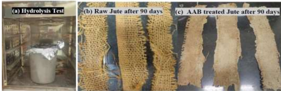
Figure 4.5. (a) Hydrolysis Test; (b) Raw Jute and (c) AAB treated jute after 90 days of Hydrolysis Test
