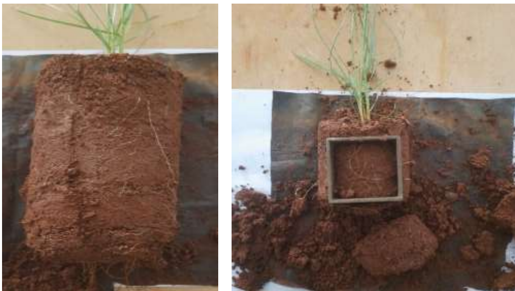
Figure 3.20. Sample collection from root-penetrated soil
