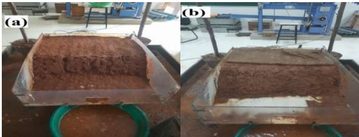
Figure 6.8. Images of a) 45° unreinforced slope; b) 45° jute reinforced slope after exposure to high rainfall for a period of 1 hr
