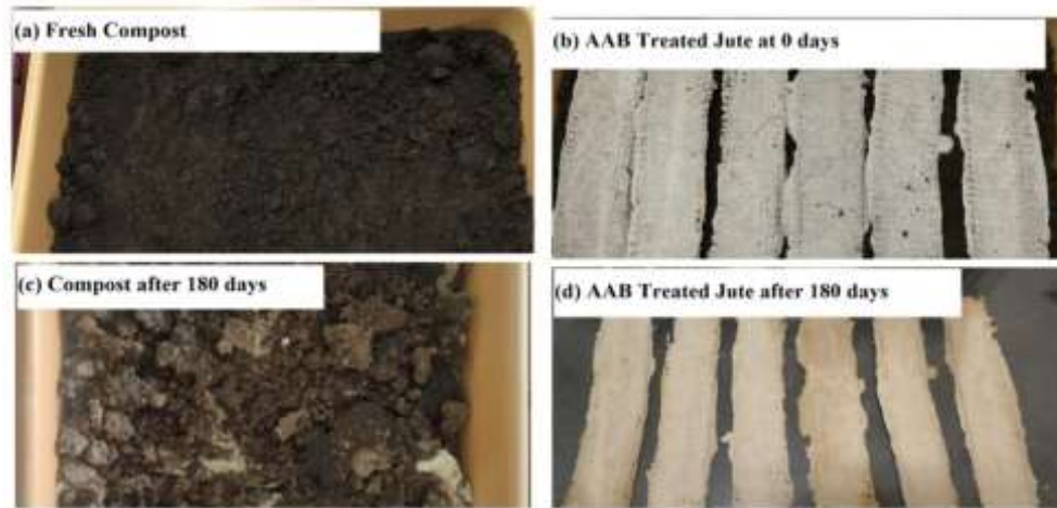
Figure 4.6. (a) Fresh Compost, (b) AAB-treated jute at 0 days (c) Compost after 180 days (d) AAB Treated Jute after 180 days
