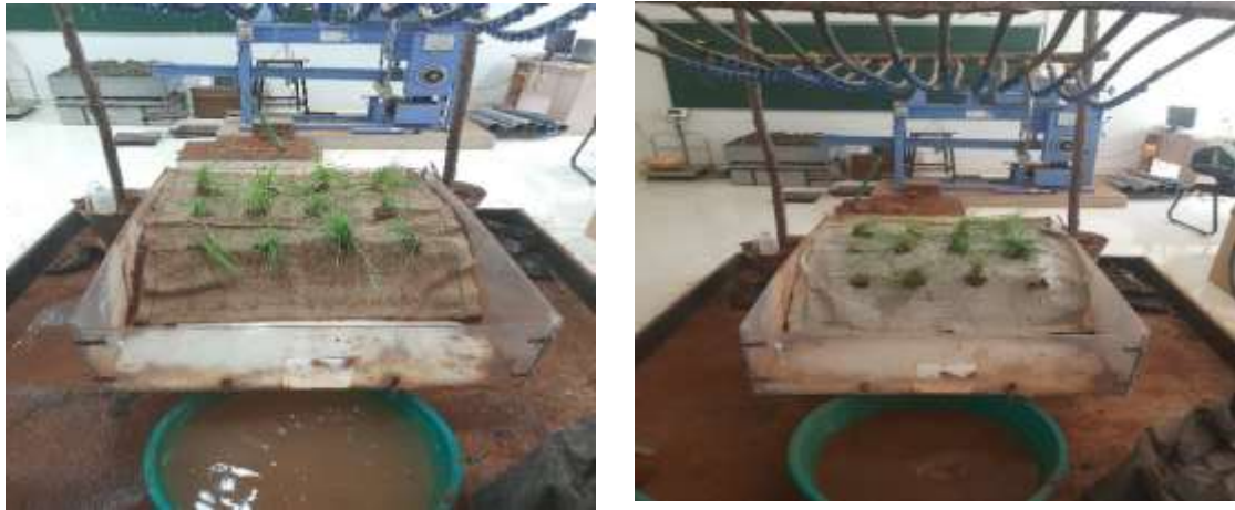
Figure 5.3. Soil erosion test for Vegetated Slope with Jute reinforcement (Left) and 0.35 AAB treated Jute Reinforcement (Right)
