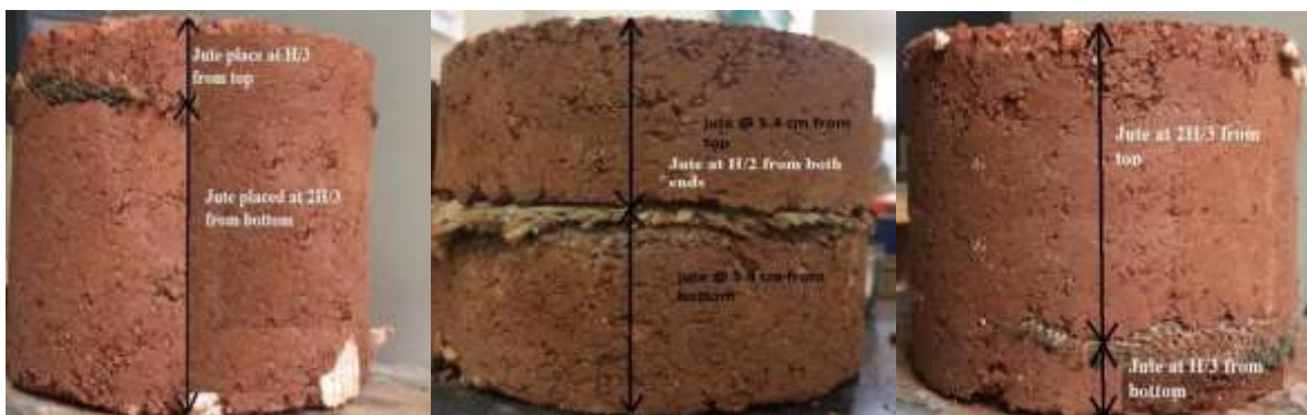
Figure 3.9. Images of jute-reinforced CBR samples at H/3, H/2, and 2H/3 positions from top
