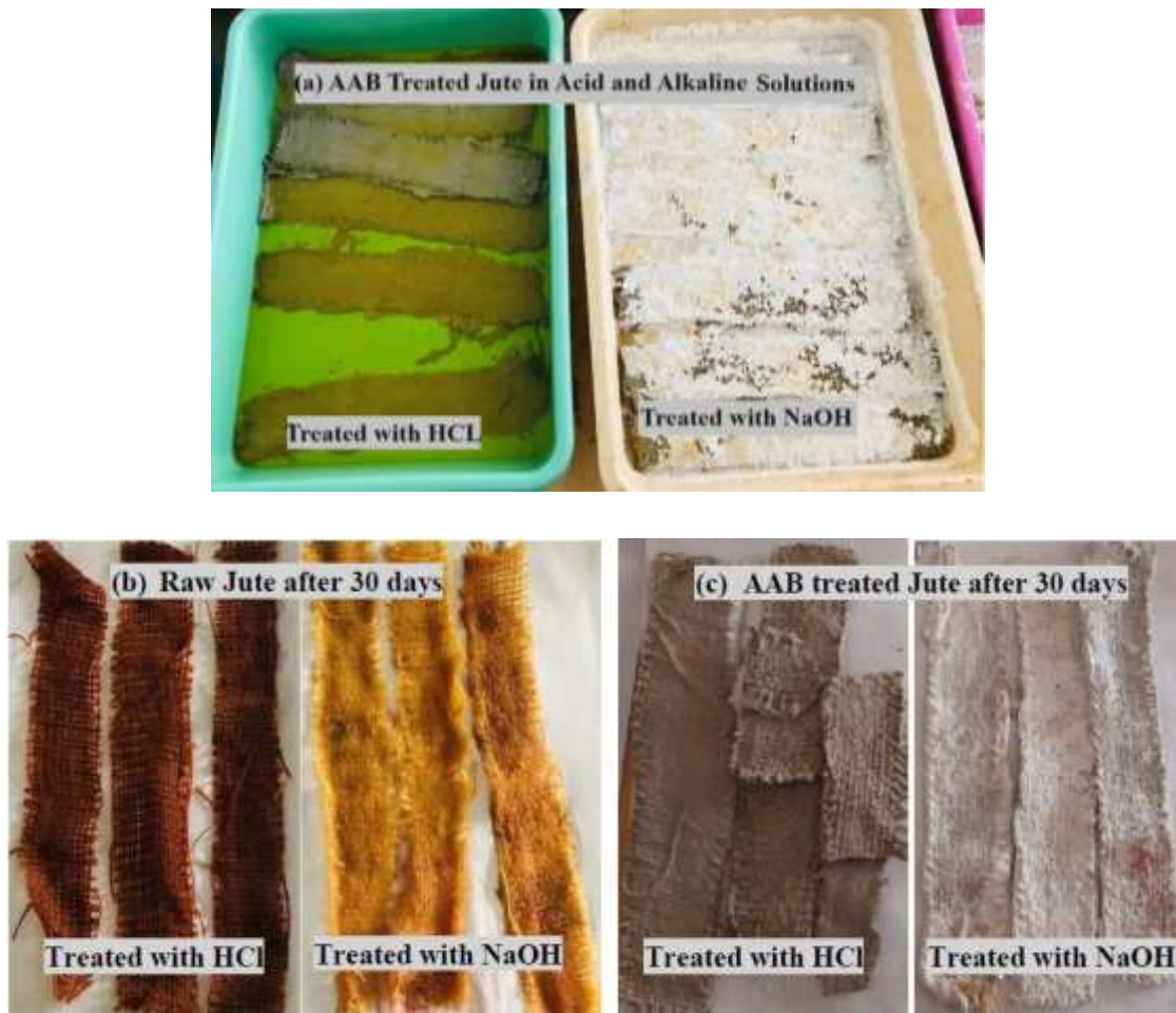
Figure 4.3. Images of (a) AAB-treated jute immersed in acidic and alkaline solution, (b) Raw Jute, and (c) AAB-treated jute after 30 days of HCl and NaOH treatment
