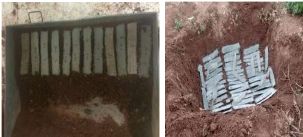
Figure 4.1. Images of JGTs in (a) Lab burial condition; (b) Field burial condition
