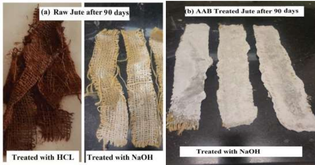
Figure 4.4. Images of (a) Raw Jute after 90 days of HCl and NaOH treatment and (b) AAB-treated jute after 90 days of NaOH
