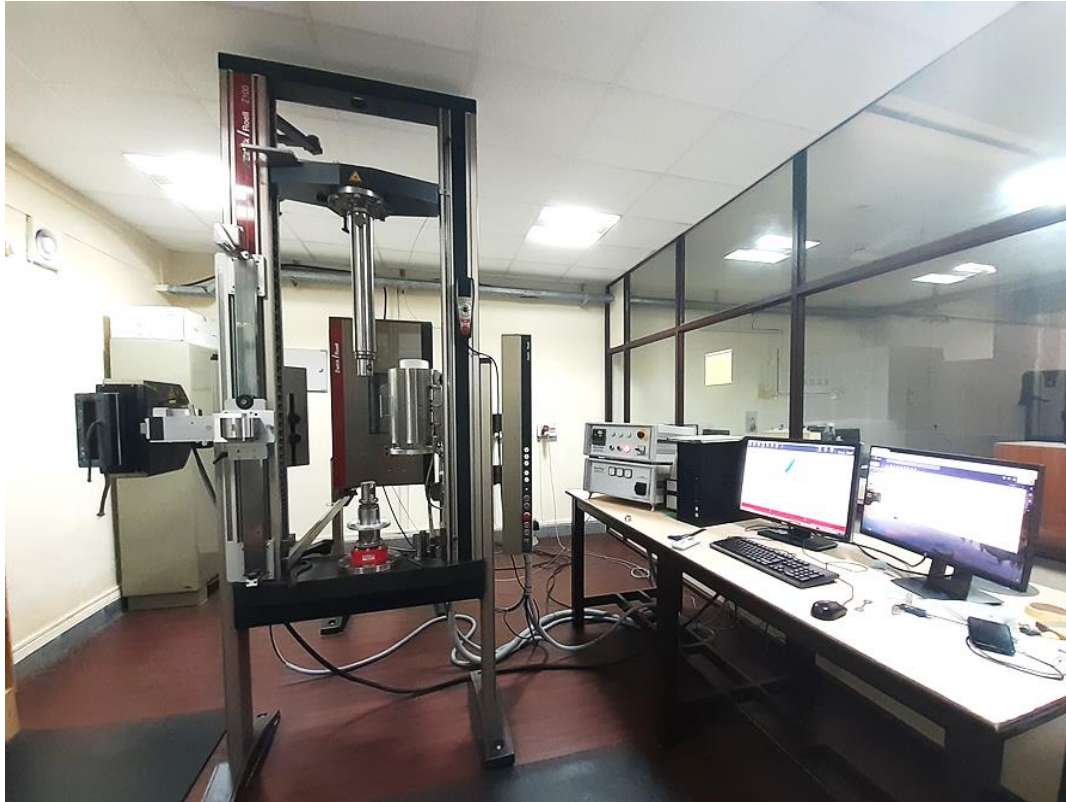
Figure 3.5 : Compression testing setup used to perform quasi-static room temperature and high-temperature tests
