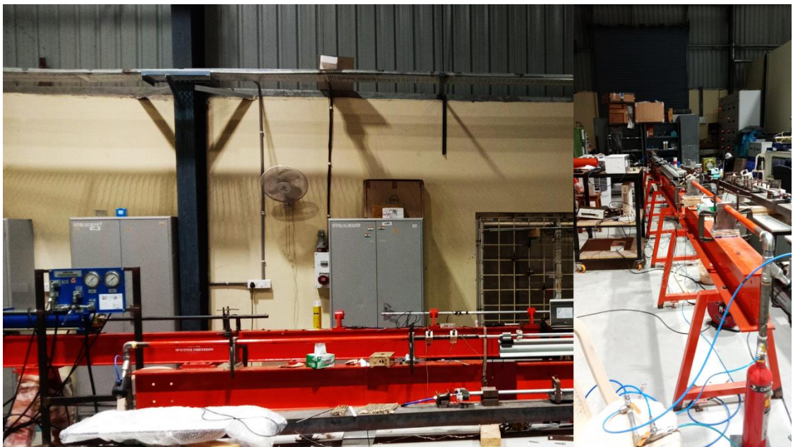
Figure 3.6 : Image of the SHPB setup used to test the SF samples.
