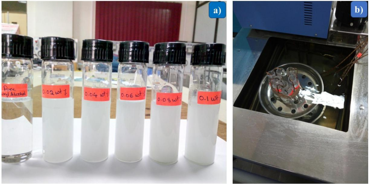
Fig. 34. a) HDP samples b) Testing the samples using TES setup.
