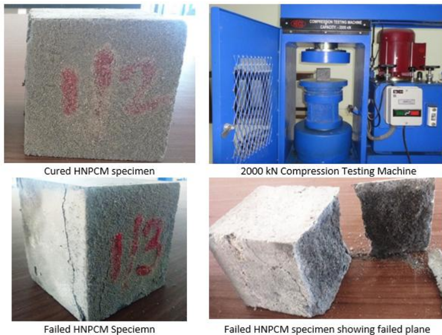
Fig. 39. Pictures showing the cube specimens during preparation, curing and post testing stages.
