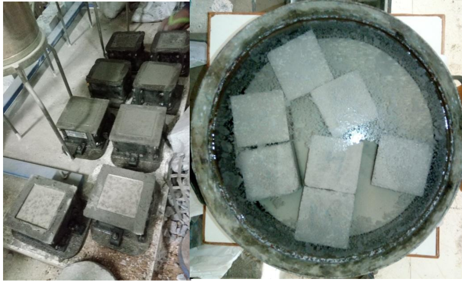
Fig. 18. HDPC preparation and curing process.
