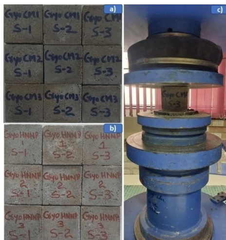
Fig. 28. a) Cryo-conditioned cement mortar cube specimens b) Cryo-conditioned HNNP based cement mortar cube specimens c) compression testing of Cryo-conditioned specimens.
