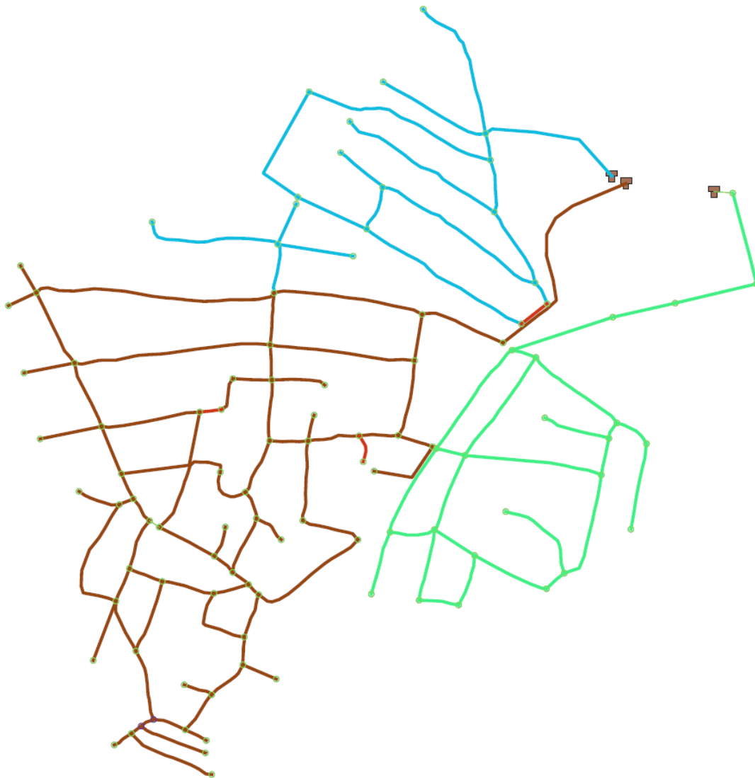
Figure 6.25 DMAs layout representing leftmost extreme point for Pamapur WDN (Green-DMA 1, Blue-DMA 2 and Brown-DMA 3)
