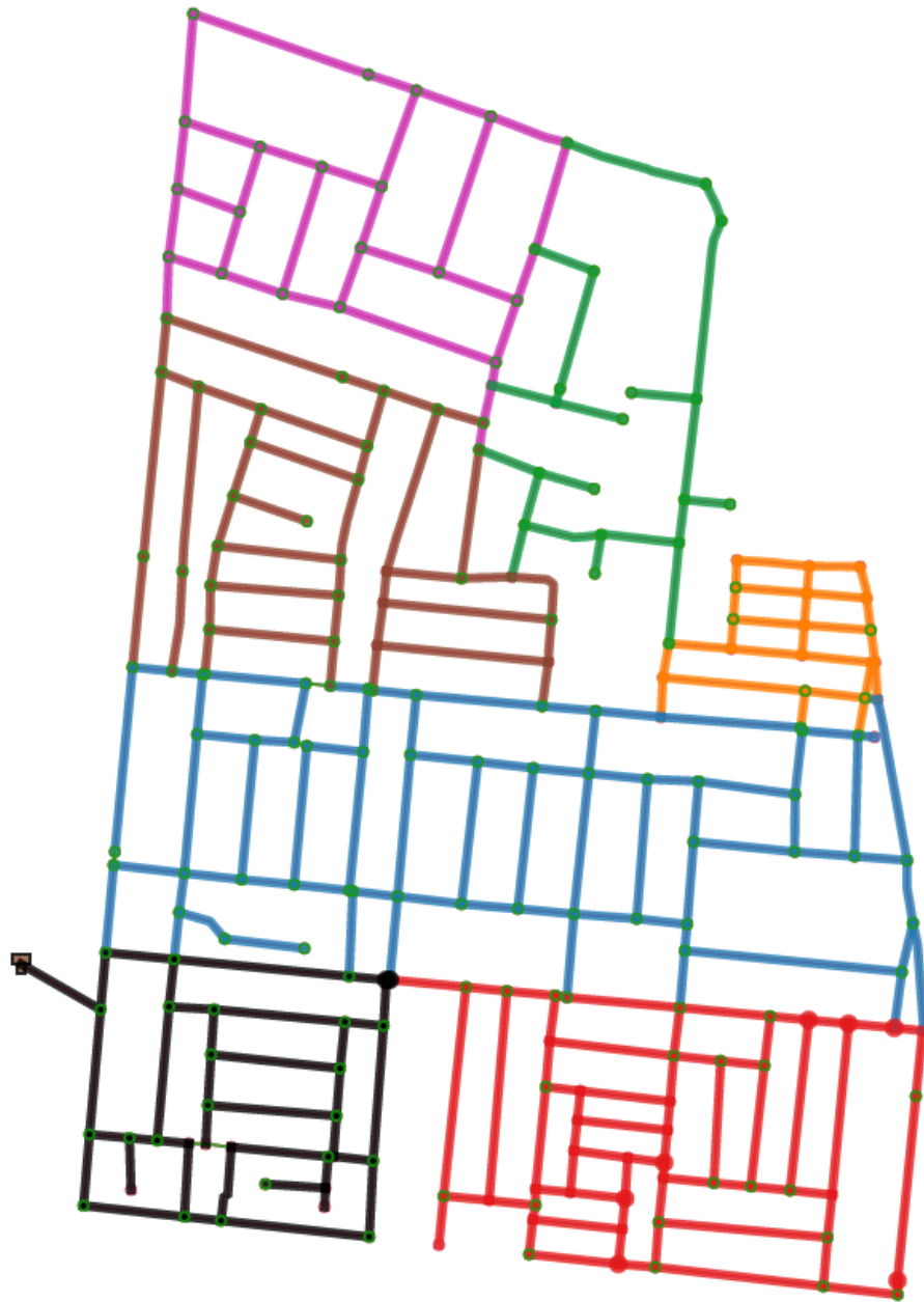
Figure 6.32 DMAs layout representing rightmost extreme point for Vanasthalipuram WDN (Black-DMA 1, Red-DMA 2, Blue-DMA 3, Brown-DMA 4, Purple-DMA 5, Orange-DMA 6 and Green-DMA 7)
