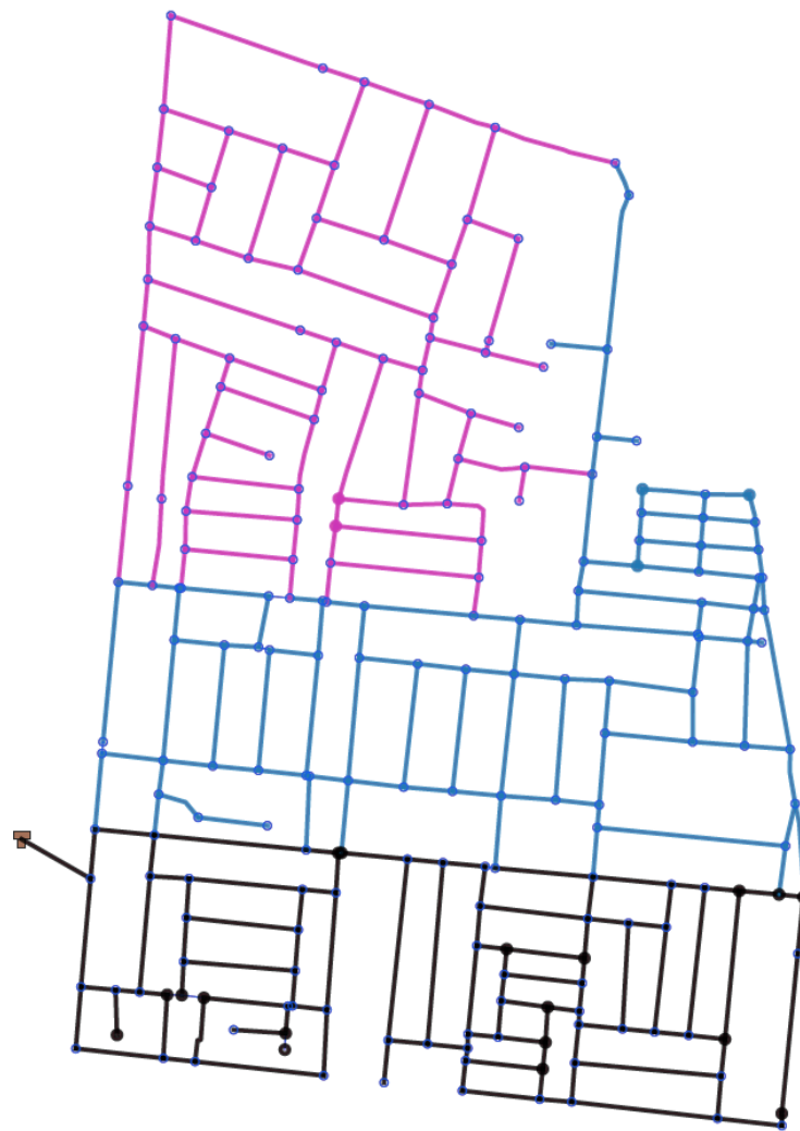
Figure 6.31 DMAs layout representing leftmost extreme point for Vanasthalipuram WDN (Black-DMA 1, Blue-DMA 2 and Purple-DMA 3)
