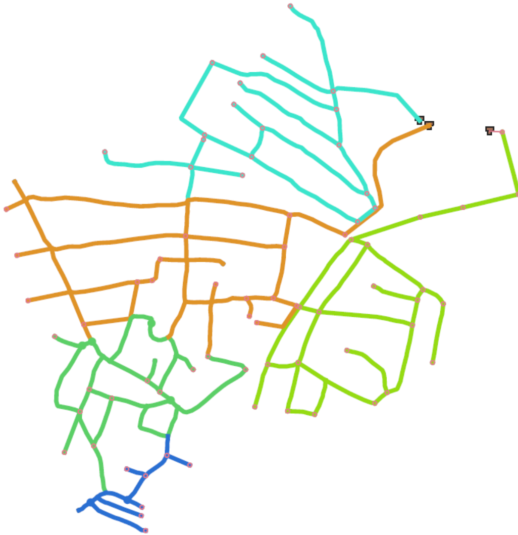
Figure 6.26 DMAs layout representing rightmost extreme point for Pamapur WDN (Light Green-DMA 1, Teal-DMA 2, Brown-DMA 3, Dark Green-DMA 4 and Blue-DMA 5)
