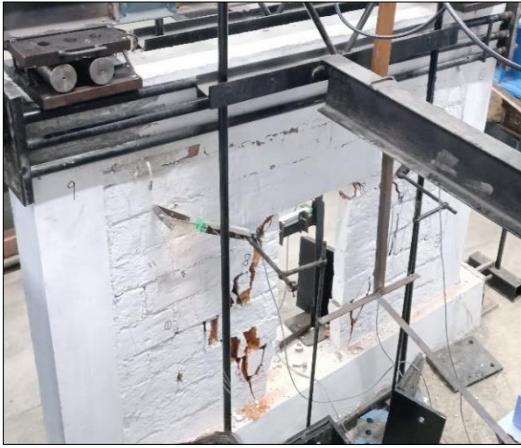
Figure 5.12(a) Initial cracks in URS specimen Figure 5.12(b) Initial cracks in DRS specimen
