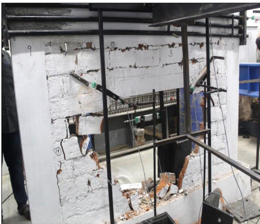
Figure 5.13(a) Final cracks in URS specimen Figure 5.13(b) Final cracks in DRS specimen
