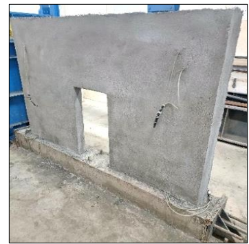
Figure 5.6(f) Specimen after placing two layers of the TRM
