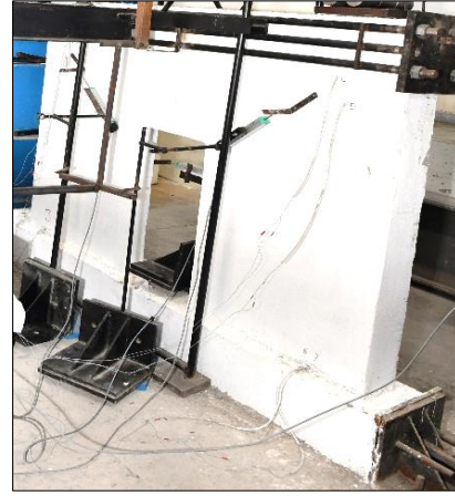
Figure 5.12(a) Initial cracks in URS specimen Figure 5.12(b) Initial cracks in DRS specimen
