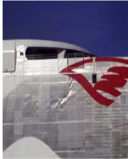
Figure 1.3: Buckling on the ship hull Structure (Lavroff et al., 2013)
