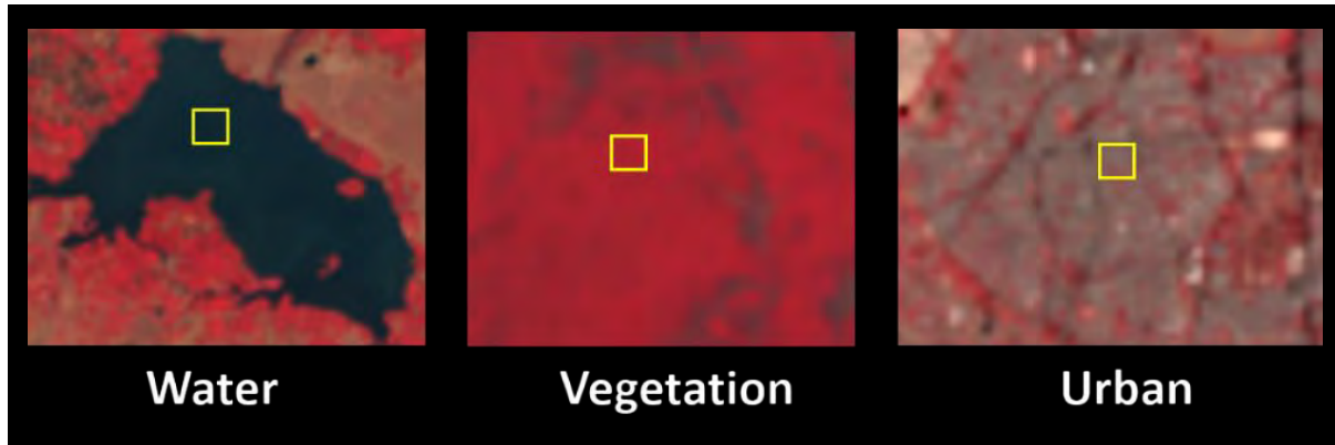
Figure-5.111. Spectral Classes in the Overlapping Region for Comparing Mosaic Reflectance (Image Layer displayed in False Color Composite)
