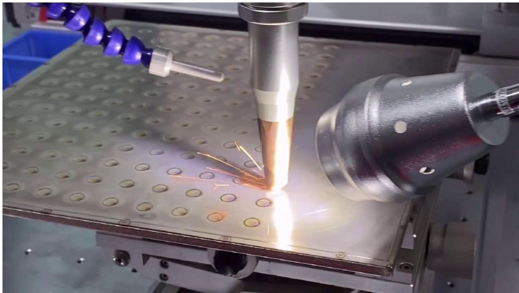
Fig. 1.3 Manufacturing of Pillow-plate heat exchanger by Laser welding operation [18]
