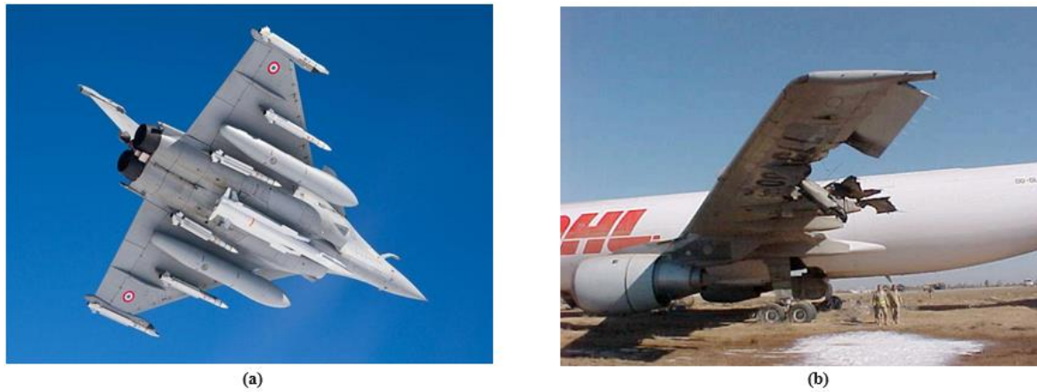
Figure 1.1. Source of c.g. variation: (a) asymmetric mass distribution (b) partial structural damage
