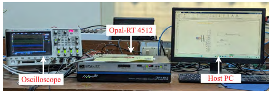
Figure 4.8: Setup for Real-Time Simulation.
