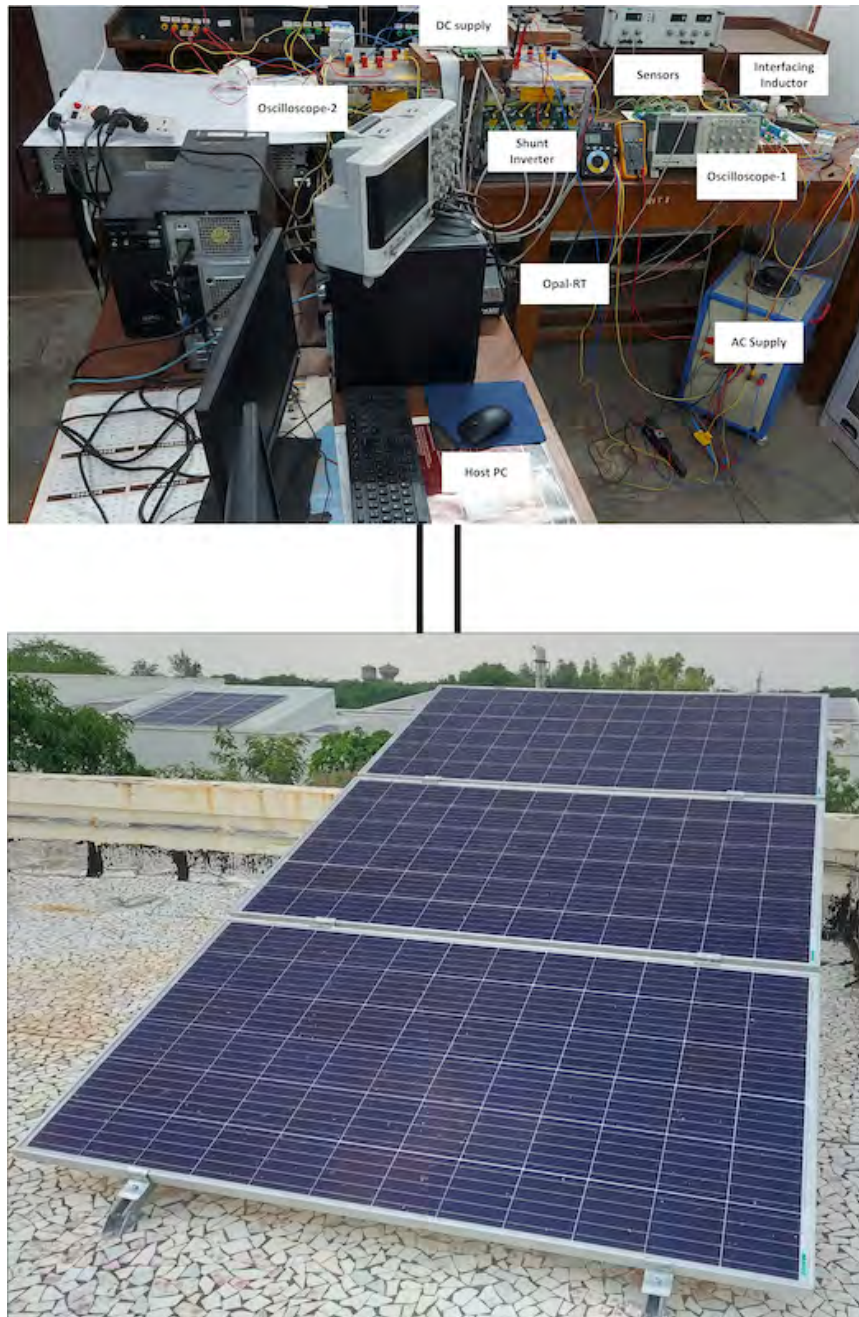
Figure 9.2: Hardware setup of PV fed shunt APF
