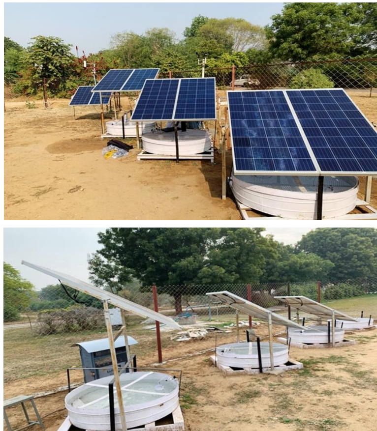
Figure. 4.1. Experiment setup of Floating Solar Photovoltaic (FSPV) system at BITS Pilani campus, India
