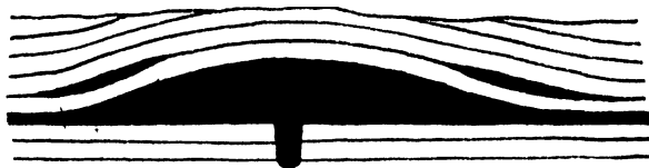
FIG. 86.—LACCOLITH PASSING LATERALLY INTO A SILL, WITH MINOR LACCOLITHS.
