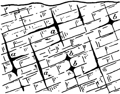
FIG. 98.—GASH VEINS, OR PIPES, AND BUNCHES IN LIMESTONE. a, GASH veins, or pipes; b, Bunches.
