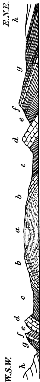
FIG. 109.—SECTION OF THE WOOLHOPE ANTICLINE. (After Murchison.)
