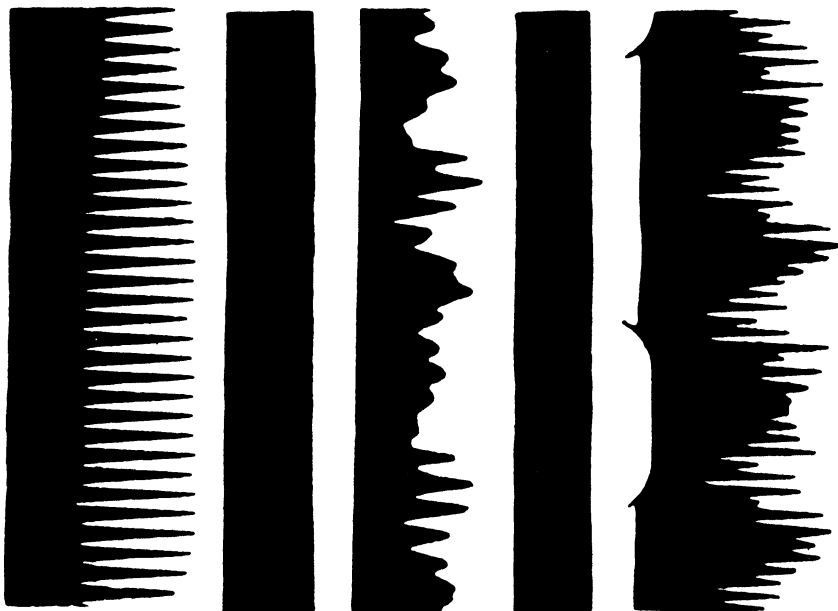
FIG. 8. Types of sound records made with R.C.A. Photophone — variable-area method. (Townsend.)
