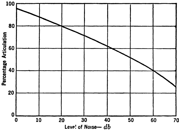
Fig. 168. Curve showing the percentage articulation of speech in the presence of a typical noise of various sound levels.
