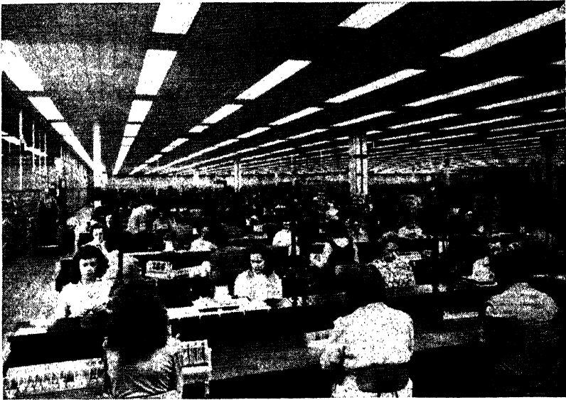
Fig 4.5. This plant was designed and built by the Austin Co. during the war for the manufacture of precision instruments and parts. The flat ceiling with acoustical tile, the diffused lighting from the recessed luminaires, and the wide spans between columns make this an attractive working area.
