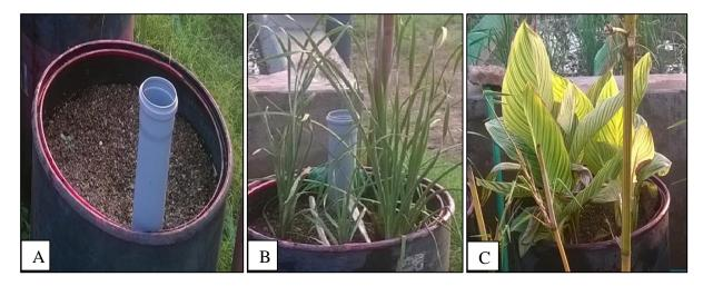
Fig 3.1: Batch scale CW in 200 l barrels. (A) Control Barrel (B) *Typha angustata* (C) *Canna indica*
