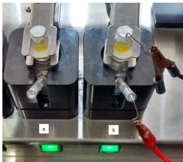
Fig.4.3. Photograph of skin permeation experiments conducted using Franz diffusion cell apparatus. a. Passive permeation of curcumin loaded liposomes. b. Iontophoresis assisted permeation of curcumin loaded liposomes.
