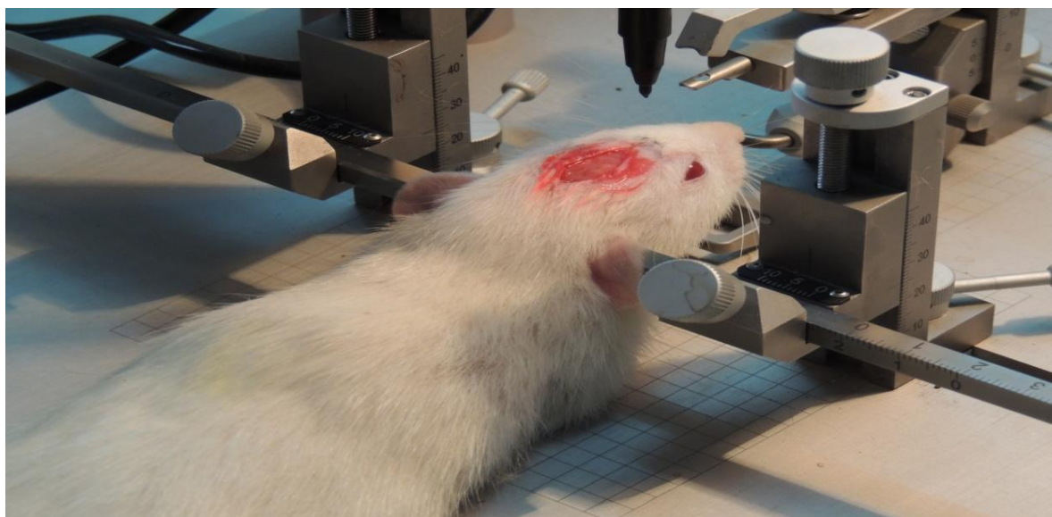
Fig.4.3 Representative Image of rat fixed in Stereotaxic frame for surgery
