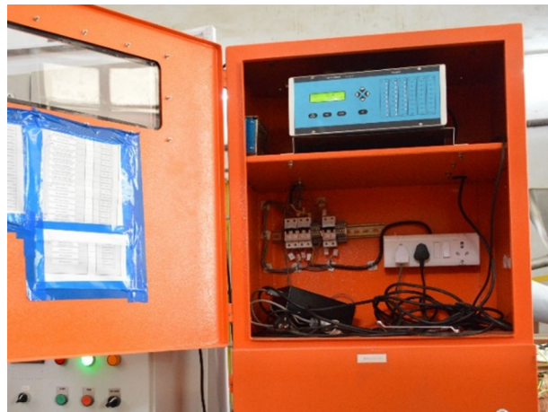
Fig. 4.16 Data acquisition system (DAQ, POLMON PL 160)
