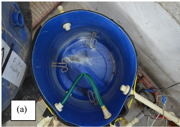
Fig. 4.11 Chiller load simulator
