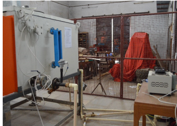
Fig. 4.11 Chiller load simulator
