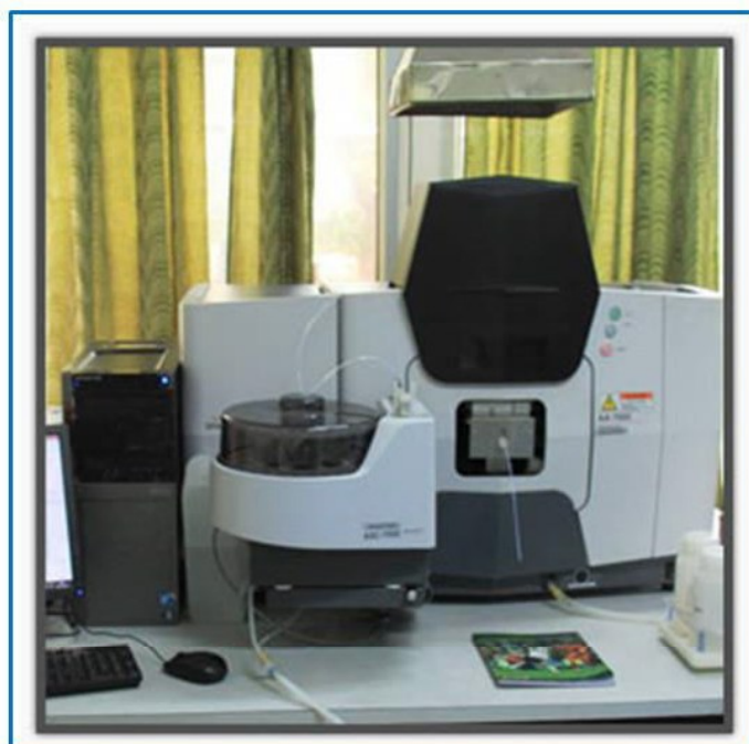
Figure 2.6: Photograph of Atomic Absorption Spectrophotometer (Shimadzu AA-7000).
