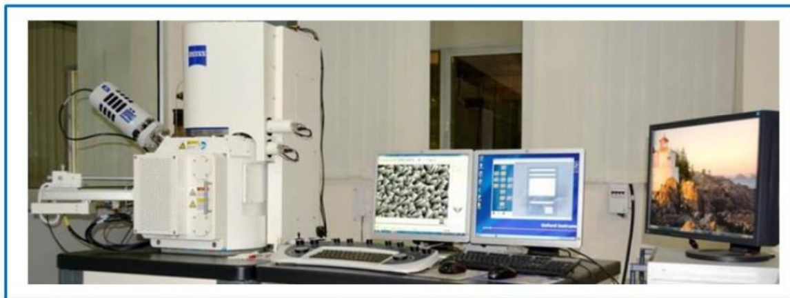
Figure 2.2: Photograph of Scanning Electron Microscope (Zeiss EVO 40).
