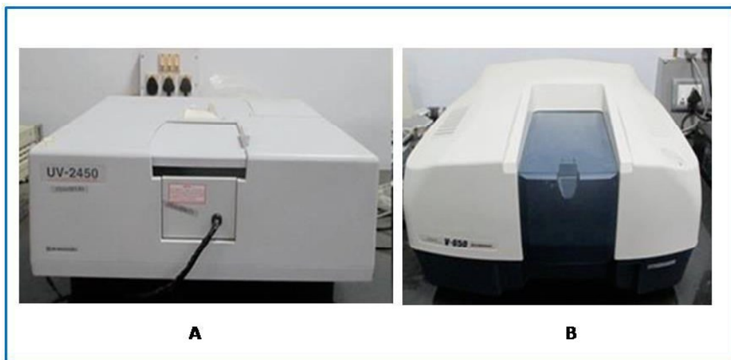
Figure 2.5: Photograph of the UV-Vis spectrophotometers (a) Shimadzu with model UV-2450 (b) JASCO with model V-650
