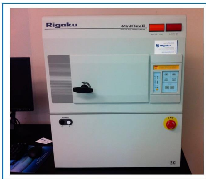
Figure 2.1: Photograph of powder X-ray diffractometer (RIGAKU MiniFlex II).
