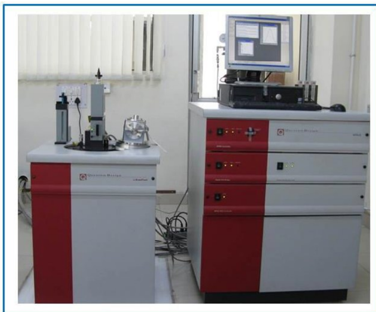
Figure 2.7: Photograph of SQUID magnetometer Quantum Design MPMS XL Ever Cool.
