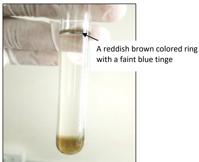
Figure 8.5: Confirmatory test for the presence of carotenoids
