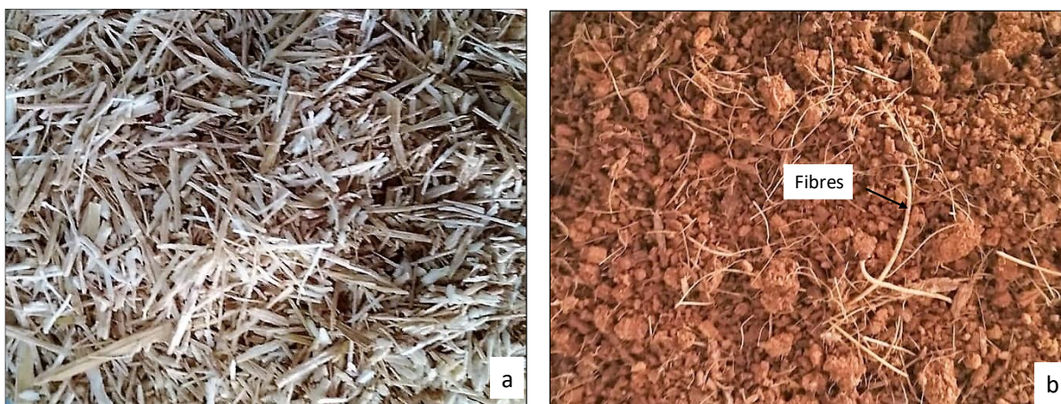
Figure 4.2: Biomass substrates with varying lignin content (a) Sugarcane bagasse and (b) Cocopeat
