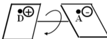
Figure 1.11: Model of a TICT excited state for a D-A molecule 231
