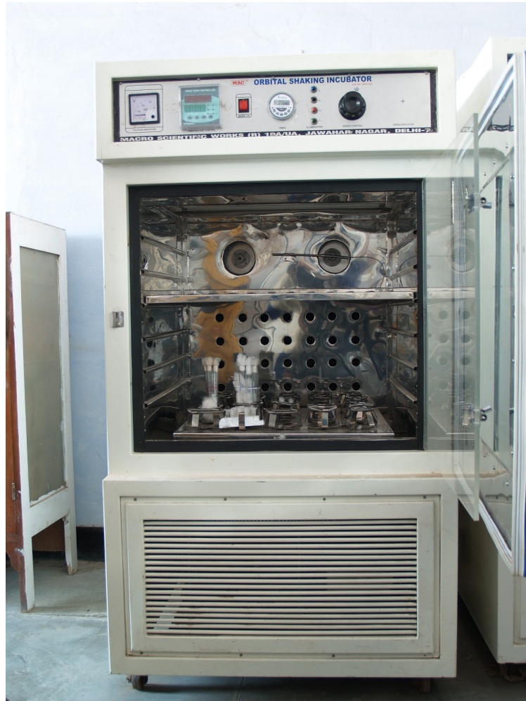
Plate 3.1. Photograph of batch experimental setup for biodegradation study
