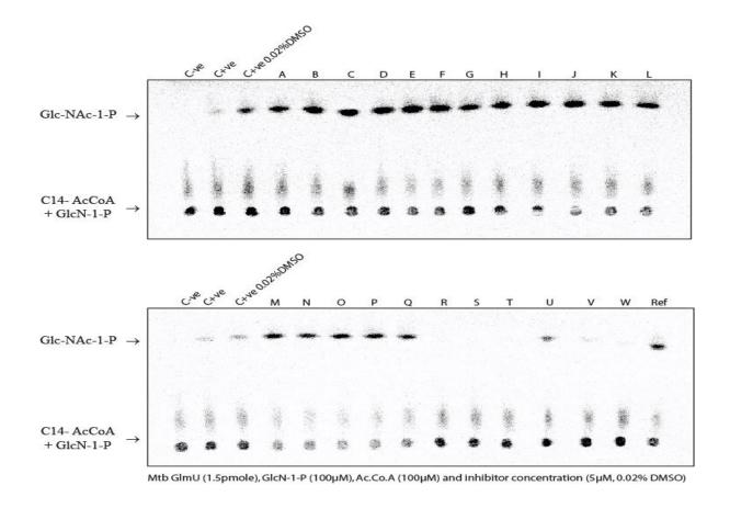
**Figure 78:** Acetyltransferase titration assay (image obtained using Phosphoimager) with a range of enzyme concentration (pmole). C-ve is negative control without enzyme. C+ve is positive control without DMSO. Spots corresponds to the product [14C] GlcNAc-1-P and unused substrate ([14C]acetyl-CoA) are indicated at  $5\mu$ M inhibitor concentration, 0.02% DMSO, 1.5pM of MTB GlmU and  $100\mu$ M concentration of AcCoA and GlcN-1-P. The compounds R, S, T, V and W showed good inhibition
