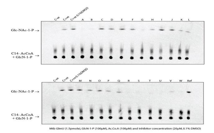
**Figure 77:** Acetyltransferase titration assay (image obtained using Phosphoimager) with a range of enzyme concentration (pmole). C-ve is negative control without enzyme. C+ve is positive control without DMSO. Spots corresponds to the product [14C] GlcNAc-1-P and unused substrate ([14C] acetyl-CoA) are indicated at 20μM inhibitor concentration, 0.1% DMSO, 1.5pM of MTB GlmU and 100μM concentration of AcCoA and GlcN-1-P. The compounds R, S, T, U, V and W showed good inhibition
