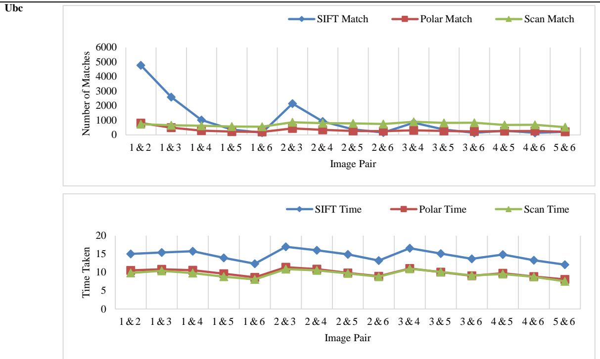
Image-set Graphs representing number of matches and time taken (in seconds) for all image pairs in each image-set of the Mikolajczyk dataset [Mikolajczyk 2007, Appendix A.1]
