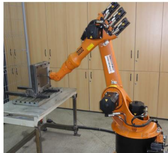
Figure 2.8. Roboforming with 6-DOF robots [19]
