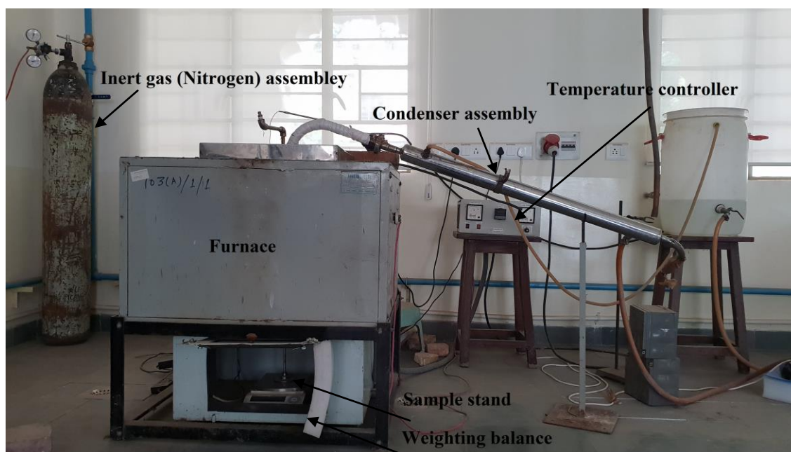
Figure I.1 Photograph of laboratory pyrolyzer setup
