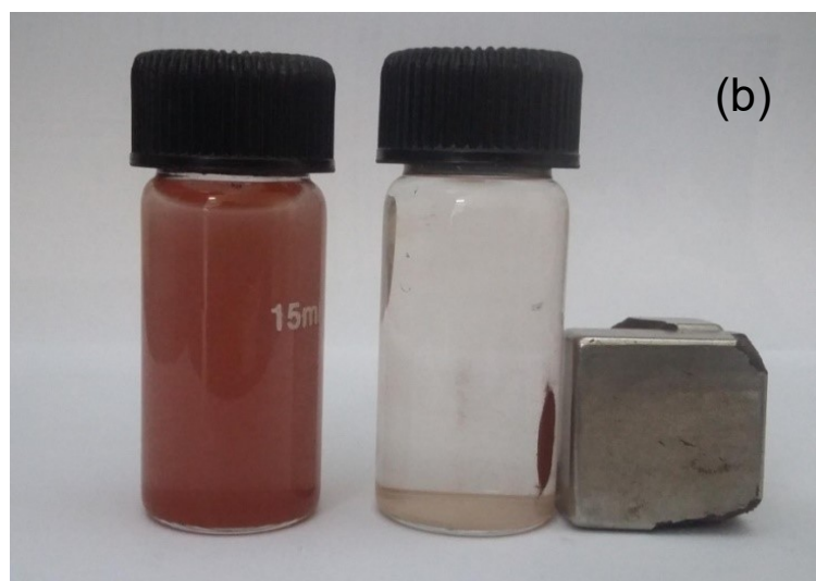
Figure 4.11: (a) Recyclability of 30% TiO 2 /Fe 3 O 4 for Cr(VI) photoreduction up to 4 cycles, (b) photograph showing the magnetic recoverability of the catalyst.
