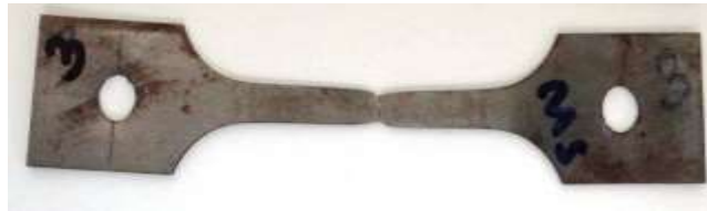
Figure 3.7: Fractured tensile specimen of IS 513 tested as per ASTM standards at room temperature
