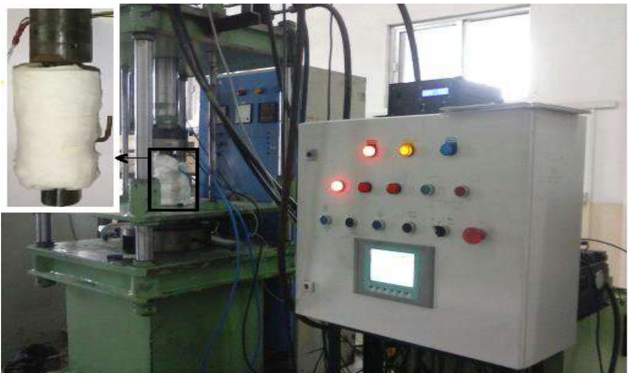
Figure 4.4: Hydraulic press setup with split punch in inset
