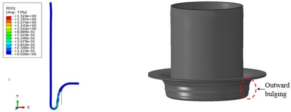
(c) Deformation predicted by FEA (at 34 mm of inversion) with an induced dimensional error
