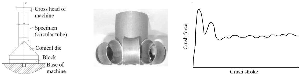
a) Tube splitting setup b) Axially split specimen c) Crush force behaviour
