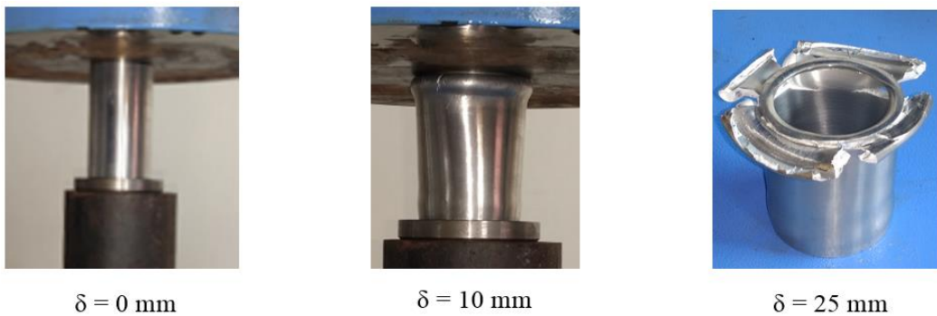
b) Progress of deformation from experiment
