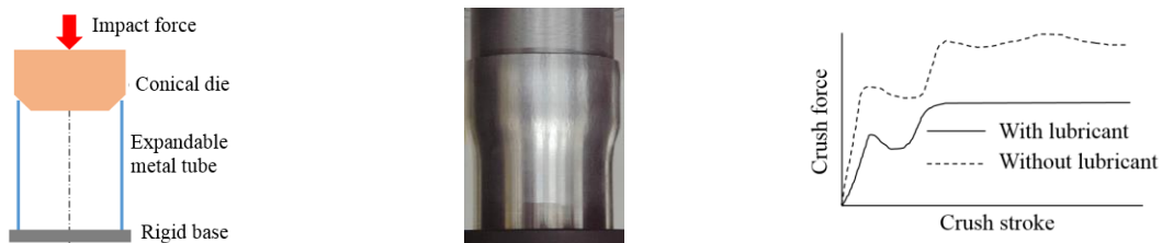
a) Schematic layout of expandable tube system b) Tube expansion process c) crush force behaviour
