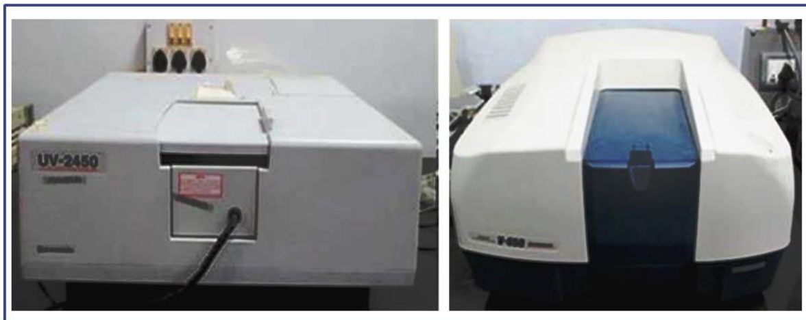
Figure 2A.2 Photograph of the UV. spectrometers, Shimadzu model UV-2450 and JASCO with model V-650
