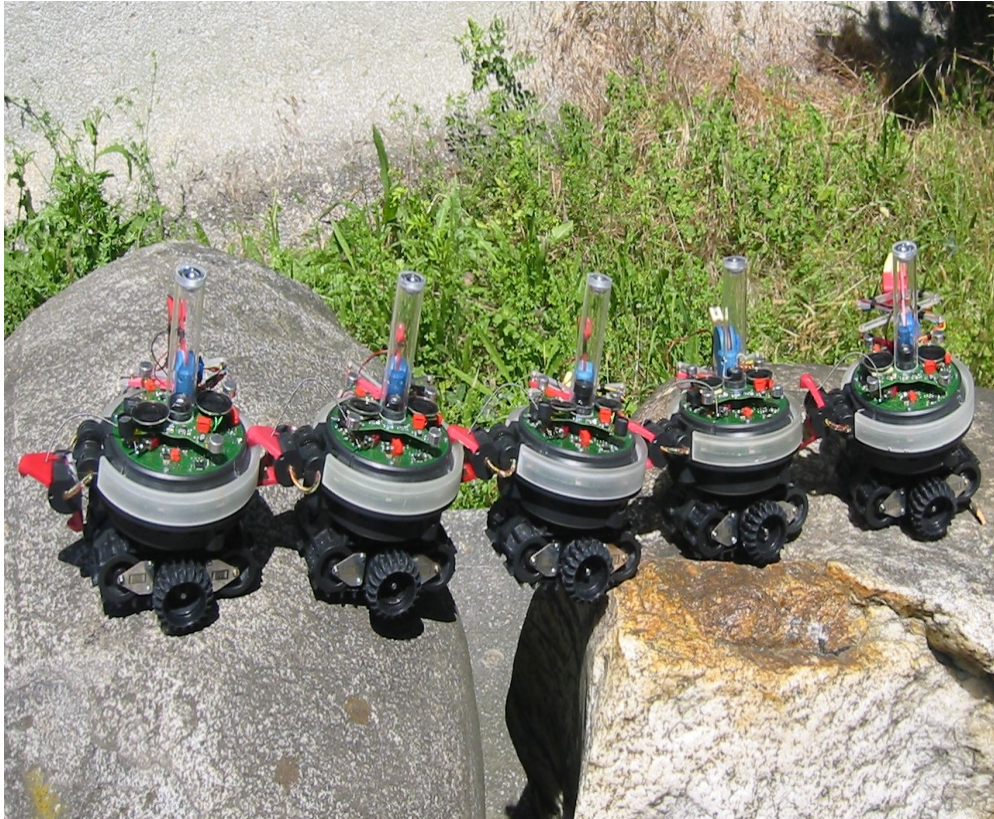
Figure 1.7. Swarm-bot modular chain structure[4]
