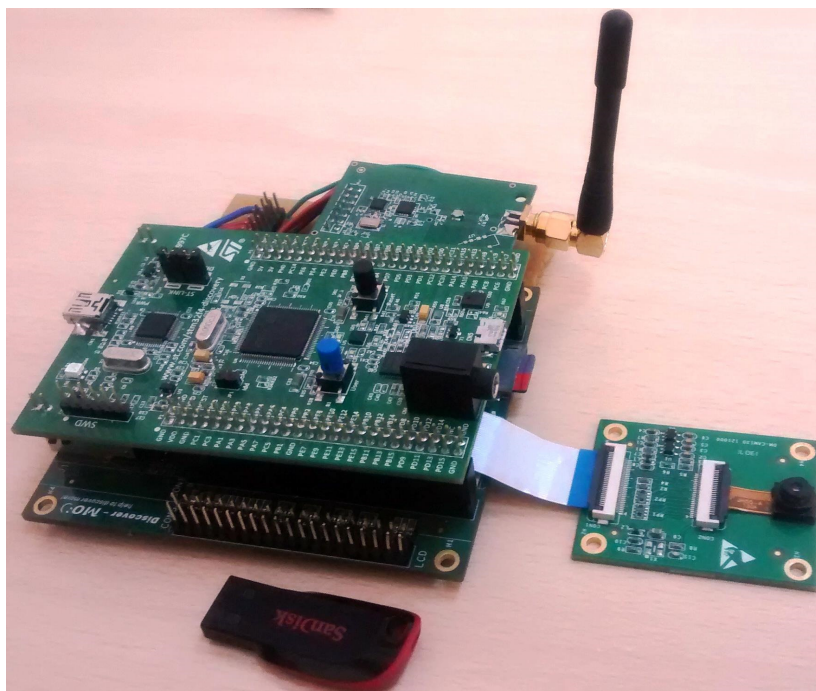
Figure 4.9. FlexEye mote prototyped using COTS components
