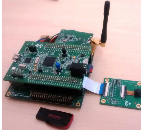
Figure 6.2. FlexEye Visual Sensor Mote
