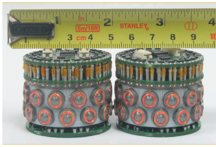
Figure 2.20. Claytronics MSRR modules[100–102]
