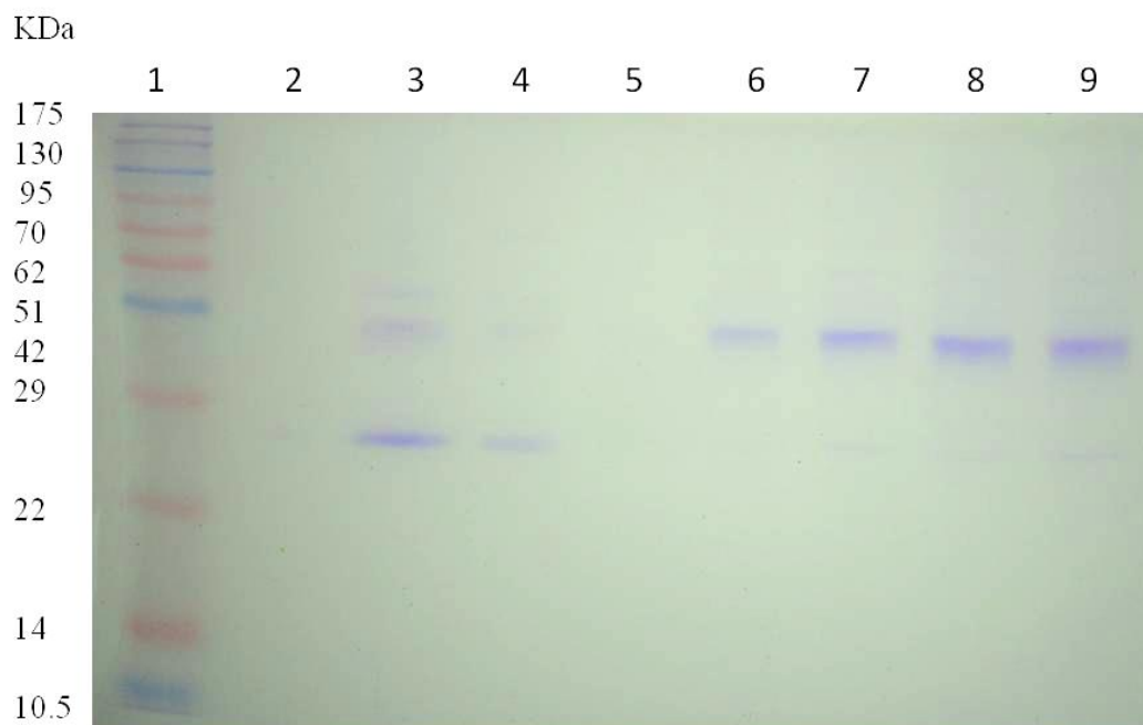
Figure 2.5: SDS-PAGE profile of tagless Sebox3 protein. Lane 1: NEX-GEN-PinkADD Prestained Protein Ladder, lane 2 and lane 5: empty, lane 3 and lane 4: tagless Sebox3 protein and GST tag and lane 6 – lane 9 purified tagless Sebox3 protein.
