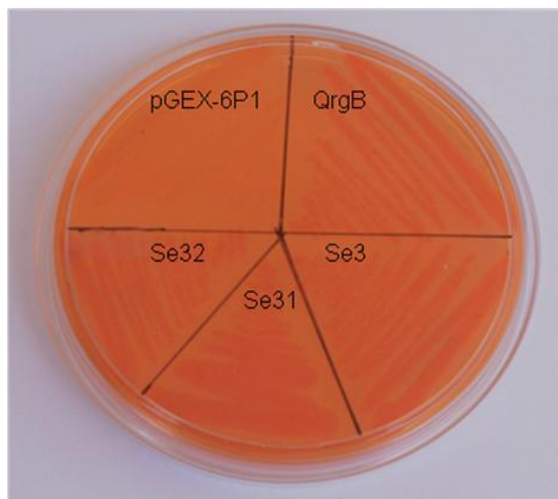
Figure 3.7: Congo Red Assay: E.coli strains with Sebox3, Sebox31, Sebox32, QrgB and pGEX-6P1 were streaked on Congo Red agar plates and incubated at 37°C. All cultures except for pGEX-6P1 acquired a red colour due to binding of Congo Red to cellulose and curli fimbriae produced in these cultures.
