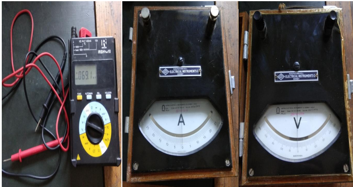
Fig. 4.17. Multimeter, Ammeter and Voltmeter used in experiment
