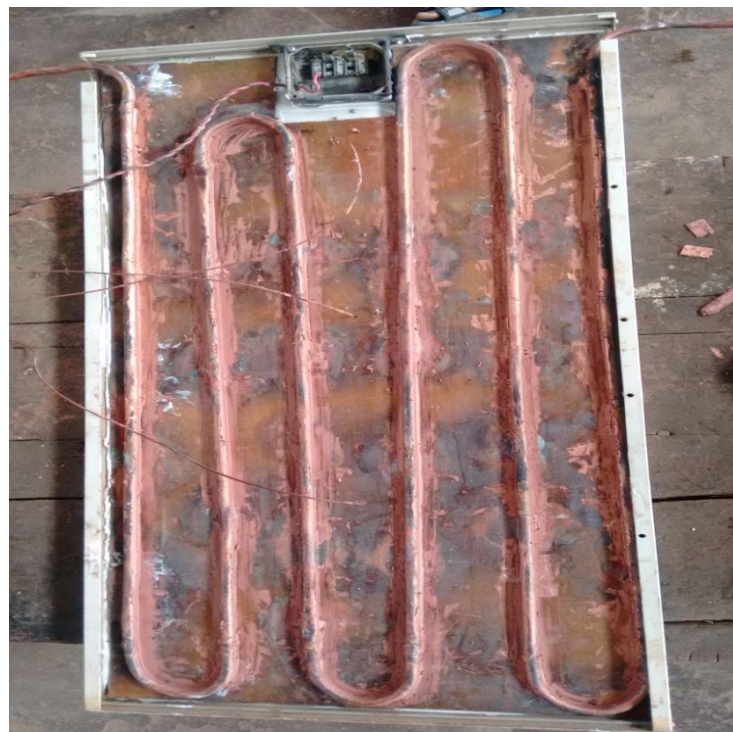
Fig. 4.3 Final tube-and-sheet PV/T water collector
