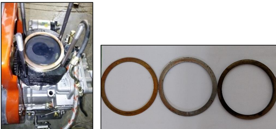
Fig. 6.1 Head gasket and compression rings for CR:11, 15 and 18
