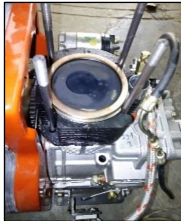
Fig. 5.2 Head gasket and compression rings for CR:11
