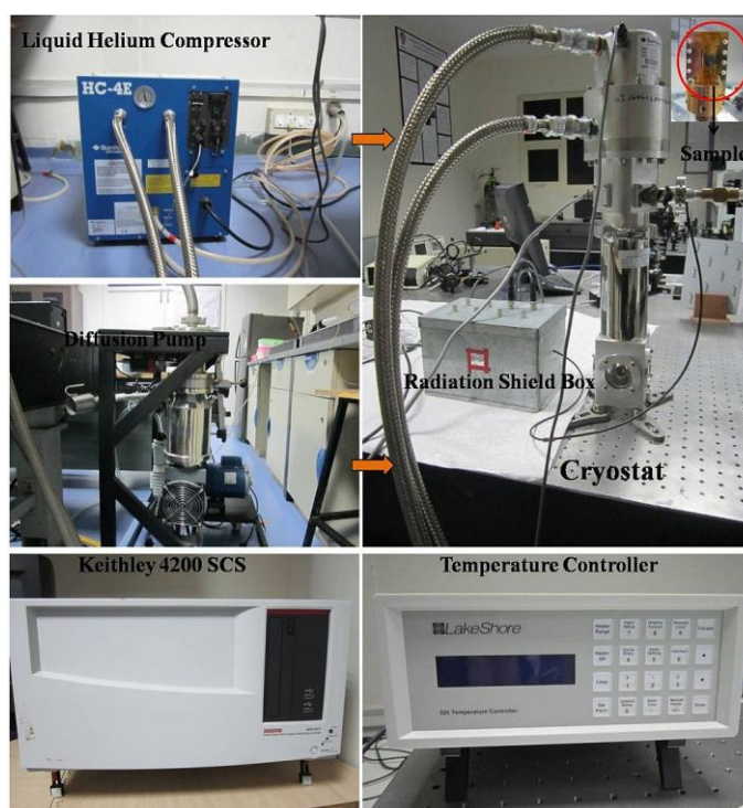
Figure 2.6: Experiment setup used for low temperature electrical transport measurement of ZnO NRs grown on ITO substrates
