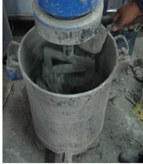
Fig 3.15 Mixing of standard ECC mixture ingredients using Hobart mixer
