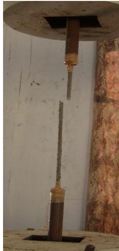
Fig. 3.29 Typical failure of CFRP bar
