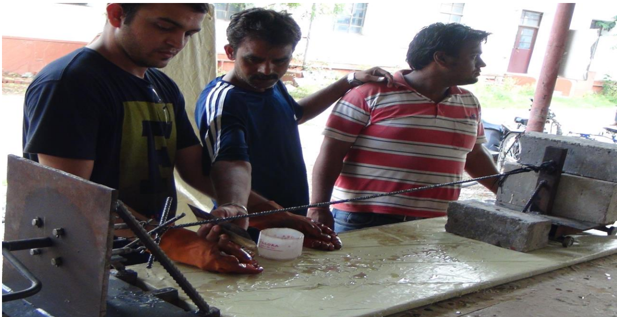
Fig. 3.27 Fabrication of CFRP bar
