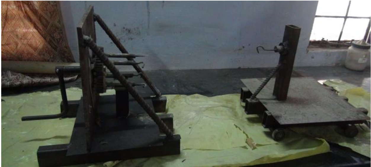
Fig. 3.26 Self-developed FRP bar manufacturing equipment
