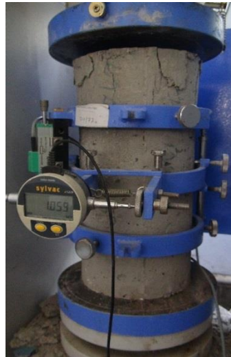
Fig. 3.16 Failure pattern of cylindrical specimen
