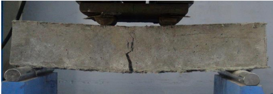
Fig. 3.23 Failure of ECC prism during four-point bending test
