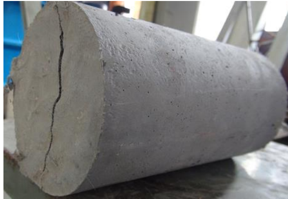
Fig. 3.19 Failure pattern of cylindrical specimen after split tensile strength test
