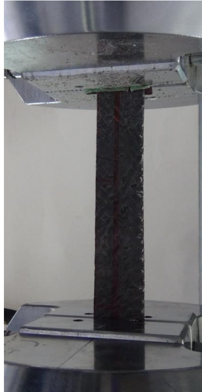
Fig. 3.24 Tensile testing of CFRP coupon
