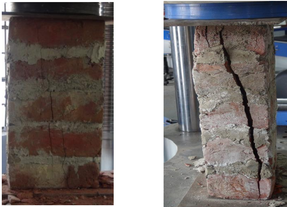
Fig. 3.11 Failure pattern of burnt clay brick masonry prism
