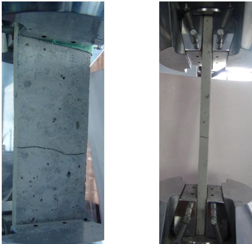
Fig. 3.20 Failure pattern of ECC coupon during tensile strength test
