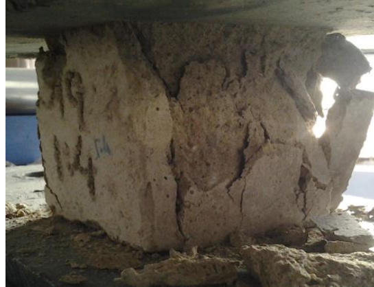
Fig. 3.5 Typical cube specimen failure of cement mortar
