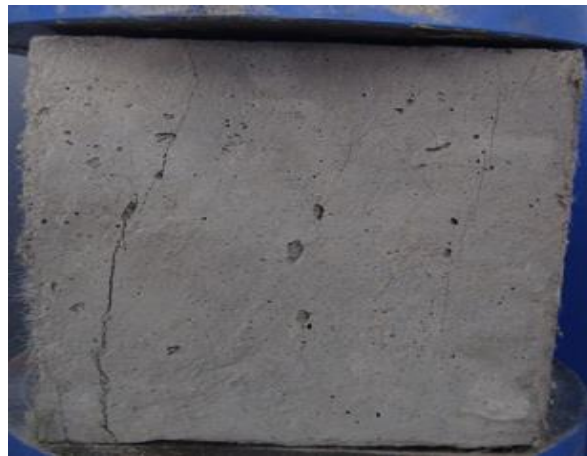
Fig. 3.18 Failure pattern of cube specimen
