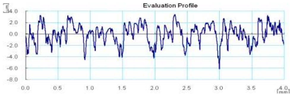
Fig. 5.6 Surface roughness evaluation profile for disc
