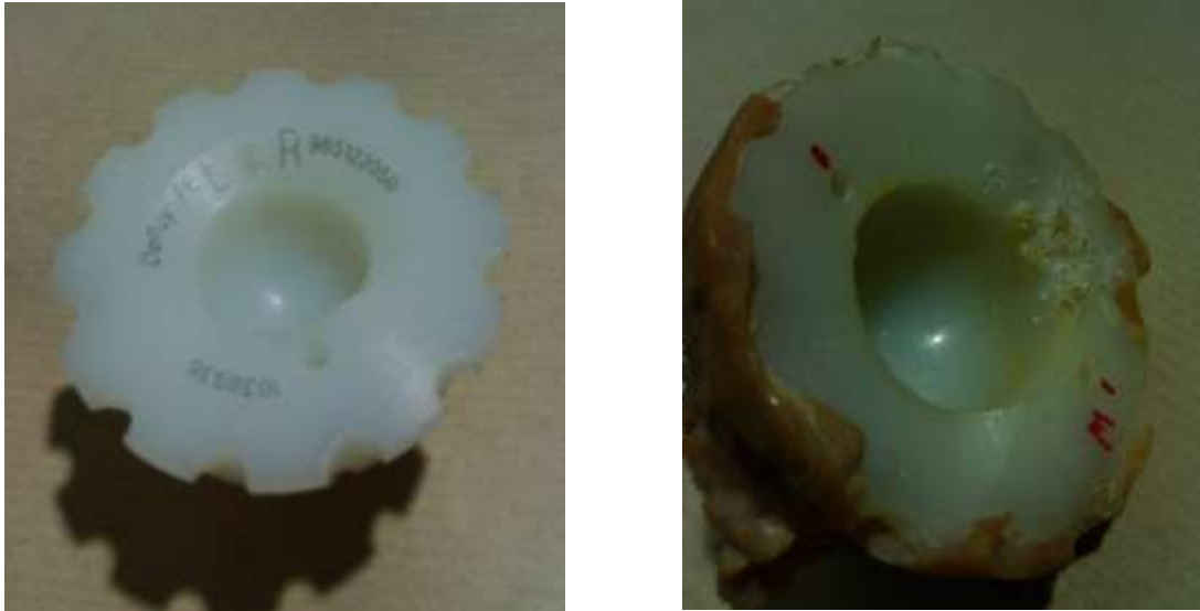
Fig. 3.1 (a) unworn cup (b) Explanted low posterior wall Charnley cup
