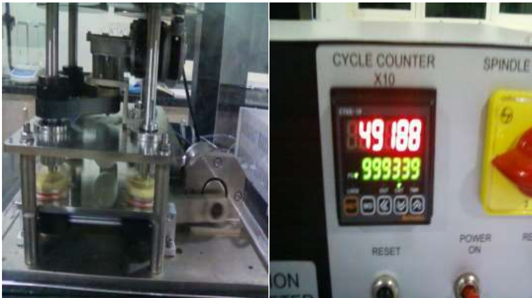
Fig. 4.3 Pin-on-plate test rig- Functional view
