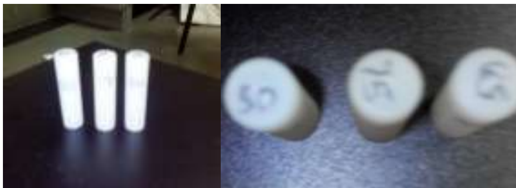
Fig. 4.1 UHMWPE Specimen pin
