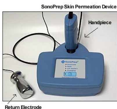
Fig.1.11. The SonoPrep ® ultrasound device. Reproduced from Mitragotri et al., 2004.
