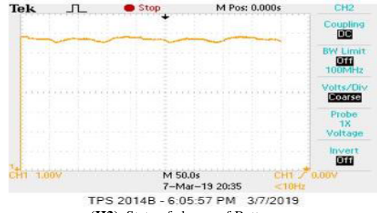
(H2) State of charge of Battery
