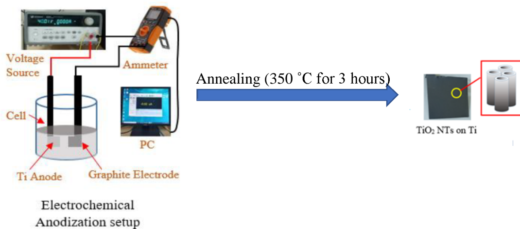
Fig.2.1. TiO 2 nanotube synthesis via electrochemical anodization route.
