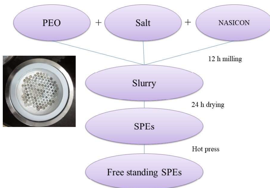
Figure 2.2 Schematic diagram of one-pot synthesis route
