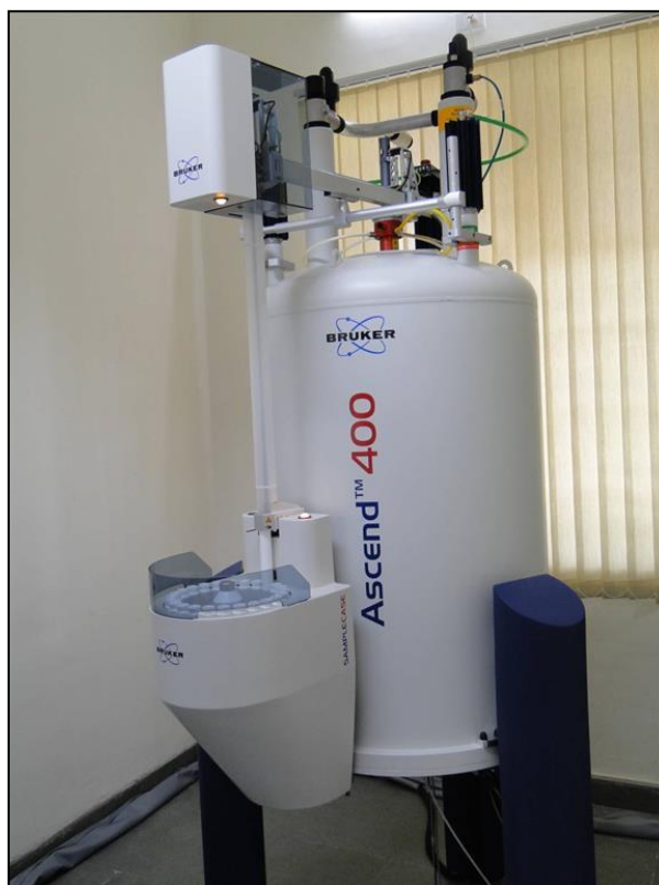
Figure 2.5: Photograph of 400 MHz NMR spectrometer (Bruker AVANCE III)
