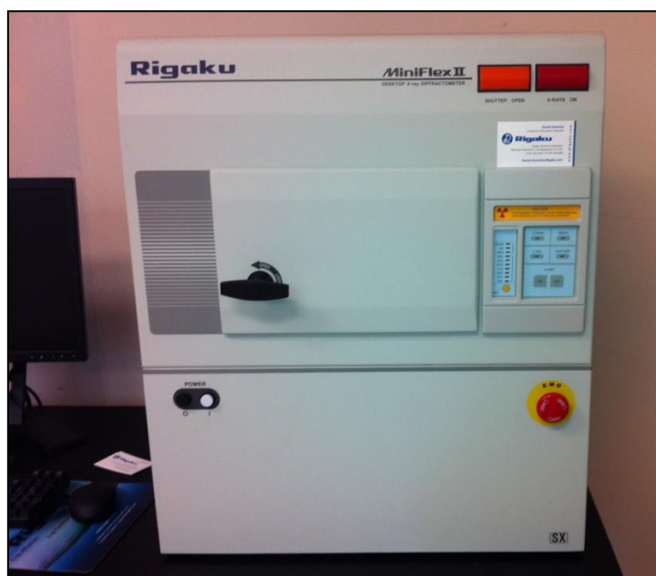
Figure 2.7: Photograph of by X-ray powder diffractometer (RIGAKU MiniFlex II).
