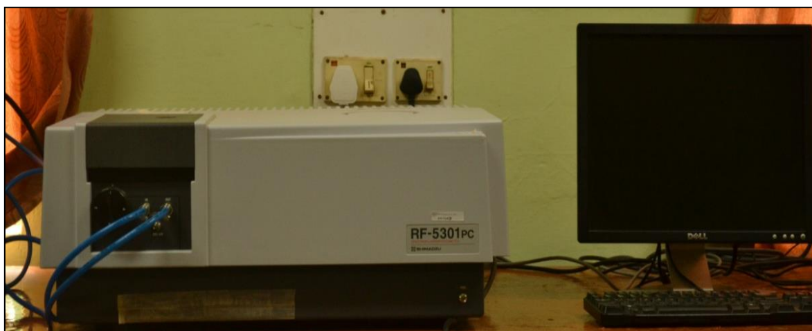
Figure 2.11: Photograph of the spectrofluorophotometer of Shimadzu model RF-5301PC.
