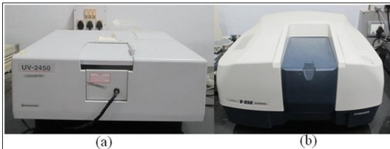
Figure 2.6: Photograph of the UV-Vis spectrophotometers (a) Shimadzu with model UV-2450 (b) JASCO with model V-650
