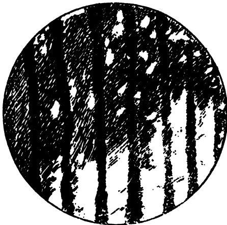
FIG. 14.—THE EFFECT PRODUCED ON A GRAMOPHONE RECORD BY PARTICLES OF A FINE PIGMENT.
