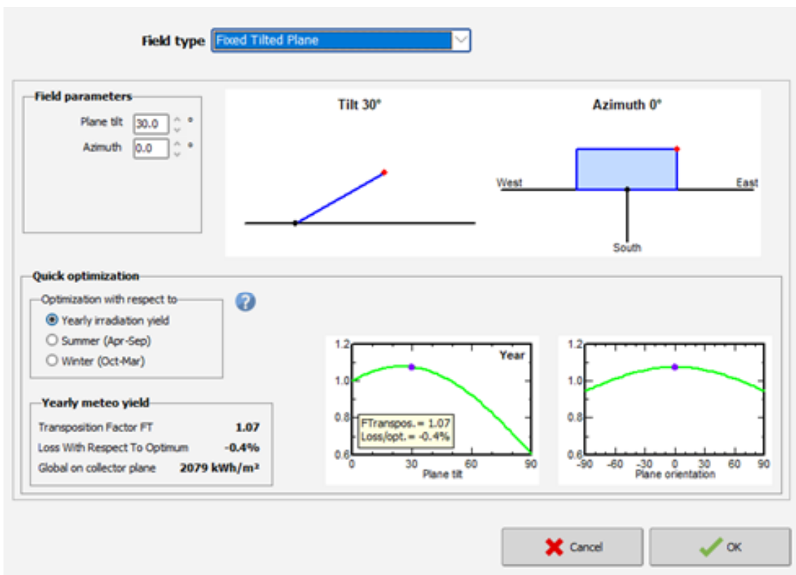
Figure 5.4 Software Report to gauge rooftop solar generation potential. Source: PVSystem Software
