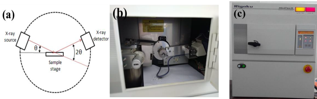
Figure 2.3: (a) Schematics view of rotating crystal X-ray diffraction method with \theta - 2\theta scan, (b) sample mounting state and rotating detector set up and (c) closed chamber X-ray diffractometer.
